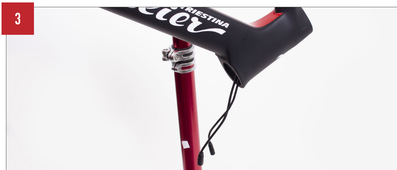
2 Exit the two battery cables from the lower hole of the head tube.
