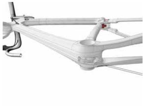
8f Pass the control cables into the special plaque (no. 8 in the «Frame» BOM), following the guides. Tighten the locking screw with a tightening torque of 3÷Nm.
