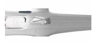
$\ensuremath{\mathbf{NB}}$  The cables are crossed in the handlebar, then run parallel inside the oblique tube and they cross again in the plate under the cage to reach correctly to the gear and derailleur.
