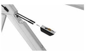
Push the cable gland plate (no. 9 in the «Frame» BOM) 8b into its seat until there is some resistance.
