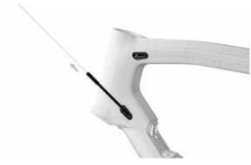
Pull the rear brake cable from the oblique tube so that  $\ \, \mathbf{1c} \,$  one end of the gland comes out.
