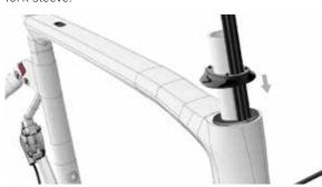
**4e** In case the top cover touches the horizontal tube: remove it, insert a micro-spacer (no. 3 in the «Parts list» BOM) making sure that the cut is wide enough to let the control cables glands and the front brake cable go through. Then put back the top cover.
