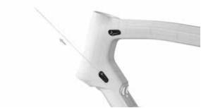
**1b** Pass the rear brake cable gland through the special grommet (no. 2 in the «Parts list» BOM).
