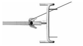
Bring the handlebar close to the stem making sure 6b that it is centred and in the correct direction.
