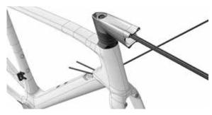
**5b** Insert the locking cartridge (no. 8 in the «Stem» BOM) between the fork sleeve and the handlebar stem.
