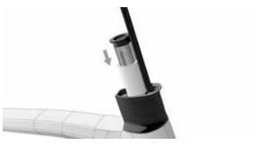
Tighten the expander (no. 5 in the «Frame» BOM) with 41 a tightening torque of 8÷10 Nm.
