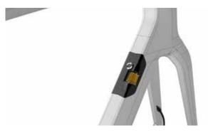
8e Let the control cables come out of the special hole under the bracket cage, making sure that they do not cross or overlap.
