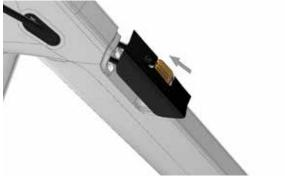
Extract the glands of the end caps and cut the excess 8c ends of the glands.
