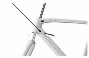
Make sure again that the glands of the control cables 4b do not cross or overlap, and pass the front brake cable through the centre between them.
