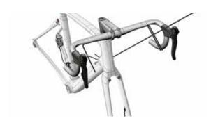
**7b** Push the controls cable glands and the glands of the front brake inside the handlebar, so that the steering can turn easily.
