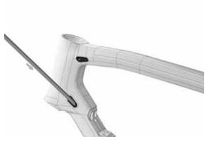
Apply the anti-vibration gland on the gland of the rear **1e** brake cable from the side of the oblique tube.
