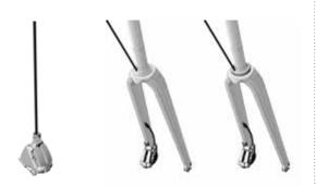
Pass the front brake cable through the special 3b grommet (no. 1 in the «Parts list» BOM). Insert the front brake cable (and corresponding gland) inside the fork so that one end comes out of the special hole on the side of the fork sleeve. Insert the bottom bearing (no. 3 in the «Frame» BOM) on the fork sleeve
