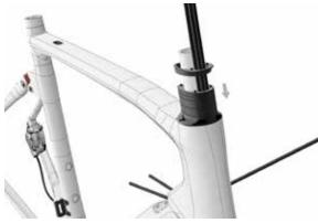
Cut the fork sleeve so that between its top border and the border of the handlebar stem, there are no more than 4 mm.
