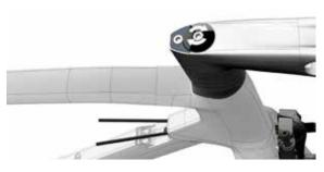
Tighten the locking cartridge with a tightening torque  $\mbox{3e}$  of  $7 \div 8 \mbox{ Nm}.$
