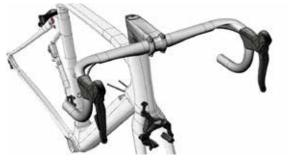
Install the front brake gland as the figure shows, 5c making sure that the steering can turn easily.
