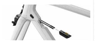
Push the cable gland plate (no. 9 in the «Frame» BOM) **7b** into its seat until there is some resistance.
