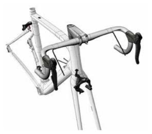
Push the controls cable glands inside the handlebar, 5b so that the steering can turn easily.
