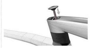
Adjust the expander adjustment screw (no. 6 in the **3d** «Frame» BOM) until the steering turns without play (apply a maximum torque of 4 Nm).
