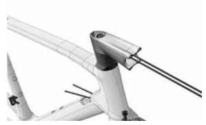
**3b** Insert the locking cartridge (no. 8 in the «Stem» BOM) between the fork sleeve and the handlebar stem.
