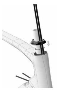
2f Insert the spacers (no. 6 and 7 in the «Stem» BOM) on the fork sleeve according to the user preferences (from zero up to a maximum overall thickness of 30 mm). Cut the fork sleeve so that between its top border and the border of the handlebar stem, there are no more than 4 mm.
