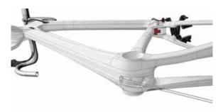
**8b** Pass the control cables into the special plaque (no. 8 in the «Frame» BOM), following the guides. Tighten the locking screw with a tightening torque of 3÷Nm.
