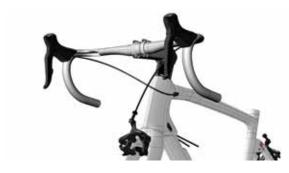
**6b** Connect the rear brake cable to the corresponding nipper, as the figure shows. Insert the gland in the rear inlet hole on the horizontal tube (no. 12 in the «Frame» BOM).
