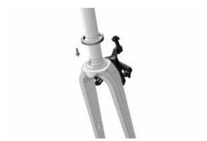
Insert the fork sleeve in the head tube from the lower **2b** hole.
