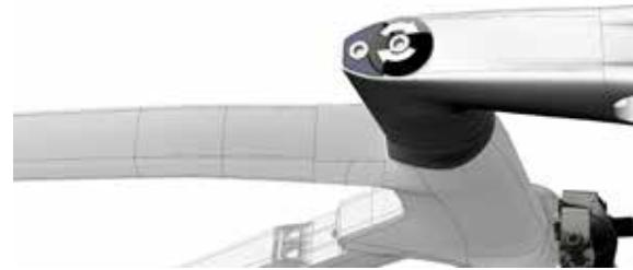
Tighten the locking cartridge (no. 8 in the «Frame» BOM) with a tightening torque of 7÷8 Nm.
