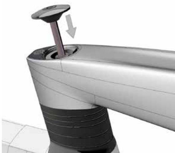
Tighten the expander adjustment screw (no. 6 in the «Frame» BOM) until the steering turns without play (apply a maximum torque of 4 Nm).
