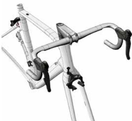
Install the front brake gland as the figure shows, **5b** making sure that the steering can turn easily.
