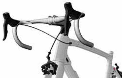
Connect the rear brake cable to the corresponding **6b** nipper, as the figure shows. Insert the gland in the rear inlet hole on the horizontal tube (no. 12 in the «Frame» BOM).
