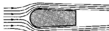
Shallower angle with sharp cut-off (Kamm tail) leaves a smaller wake and less drag.
