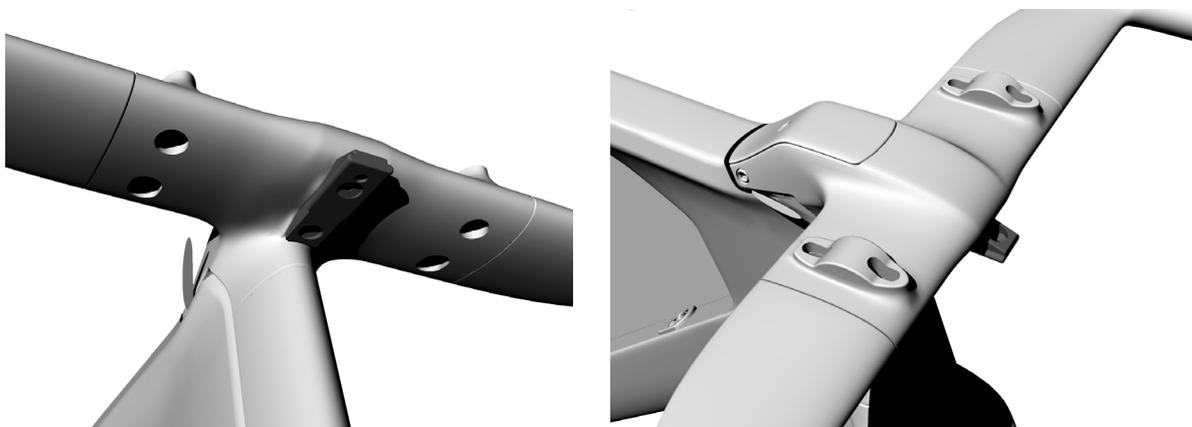
**3 FISSARE LA BORRACCIA ALLA GUIDA, AVVITANDO LA VITE NEL FORO FRONTALE.**
