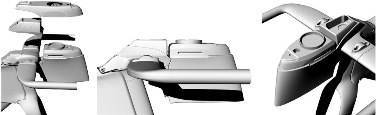
**5** POSIZIONARE LA COVER DELLA BORRACCIA E FISSARLA PER MEZZO DELL'APPOSITA VITE
