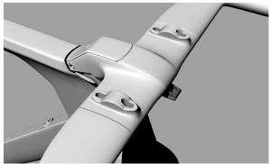
PUT THE BOTTLE CAGE TO THE TRAIL, TIGHTENING THE SCREW ON THE CENTRAL HOLE
