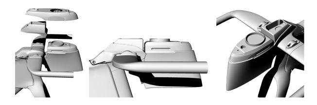
PUT THE COVER ON THE BOTTLE CAGE AND FIX IT WITH THE PROPER SCREW
