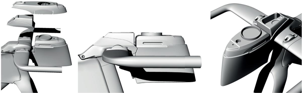
**5** PLACER LA COUVERTURE DU BIDON ET LA FIXER AVEC LA VIS APPROPRIÉE
