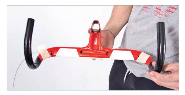
Take the bar/cable assembly & thread the inner cable that emerges from the RIGHT side of the bar into the LEFT hand outer cable. Thread the inner cable that emerges from the LEFT side of the bar into the RIGHT hand outer cable. As can be seen in the images, when correctly installed the outer cables will cross in under the centre of the ALABARDA stem.
