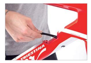
Keep applying pressure to the outer cables whilst turning the handlebars to the full limits of travel both clockwise & anti-clockwise.
