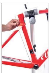
Position the DOWN TUBE COVER PLATE on the frame and fix in position with the screw.
