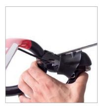
Secure the shifter levers in the desired position. Using the torque recommended by the shifter manufacturers.
