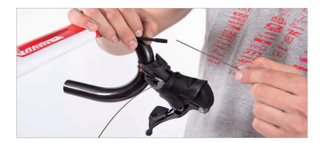
Thread the inner cables through the installed inner cables.
