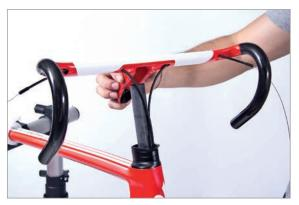
Gently push the outer cables into position inside the stem cavity as shown.
