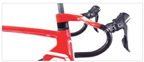
Withdraw the cables from the outer cables so the inner cables are well clear of the lower ends of the outer cables fitted inside the down tube.
