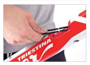
Release the pressure & cut the outer cables at the marked positions. With no pressure applied, the ends of the outer cables should line up with the end of the down tube cavity as shown. Fit the gear outer cable end caps.
