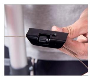
The FD / RD gear inner cables are threaded into the frame through the down tube apertures as shown. Again, FD cable on the right & RD cable on the left.
