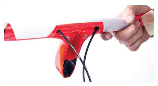
Carefully install the ALABARDA into position on the steerer whilst ensuring the outer cables remain in the correct place. Ensure that all 4 ends of the outer cables are outside the frame / bar & remove the inner gear cables.
