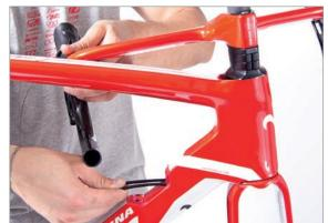
When the gear cables are in the correct position, mark the position in the centre of the down tube cavity as shown.
