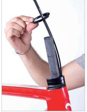
This image shows the correct assembly of the TOP SPACER & BOTTOM SPACER.
