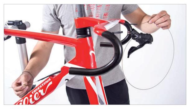
Fit the shifters. We suggest fitting the outer cables BEFORE fixing the levers in the  $\,$  desired position.
