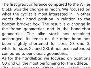
The main changes affect drop, reach, and handlebar tilt angles. In particular, those of the handlebar stem in relation to the fork sleeve, which range from 7.5 to 10.5 degrees. We paid particular attention to the distance between the bottom bracket and the high hand rest on the handlebar, which we at Wilier have christened as point CO or ACCU-FIT.
