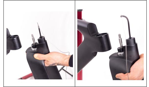
5. Insert the rear brake hose from the hole placed on the left side of the chainstay. Slide the brake hose onto the frame until it comes out the headtube, as shown in the picture.
