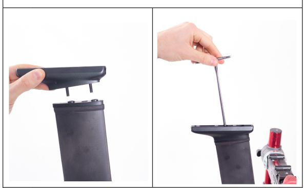
27. Insert the threaded pin into the seat post rail hole. It will be used to secure the seat clamp.
