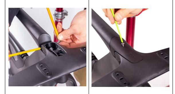
16. Place the front derailleur mount plate into its seat, tightening the two bolts to 3 Nm (each plate mount uses the same torque values).
