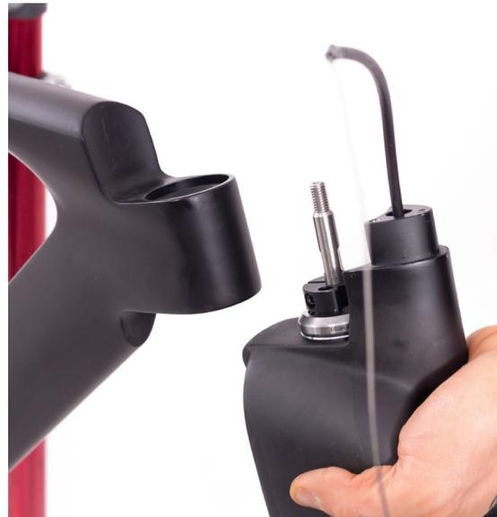
5. Insert the rear brake hose from the hole placed on the left side of the chainstay. Slide the brake hose onto the frame until it comes out the headtube, as shown in the picture.
