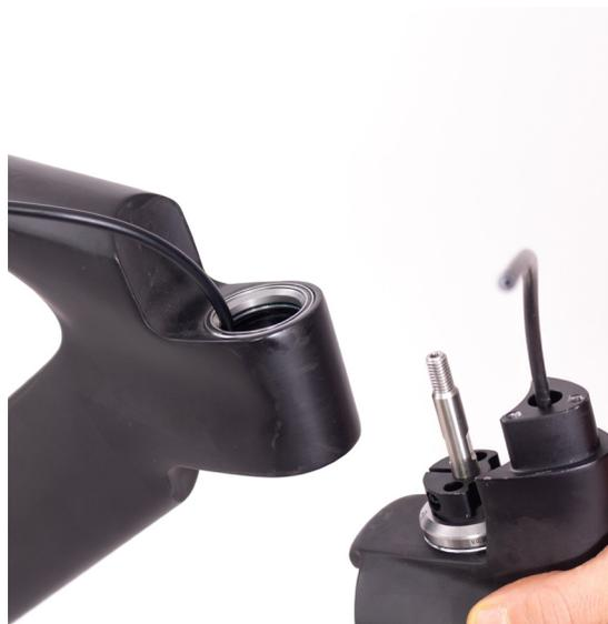
7. Insert the fork into the headtube making sure the bearings are properly seated.
