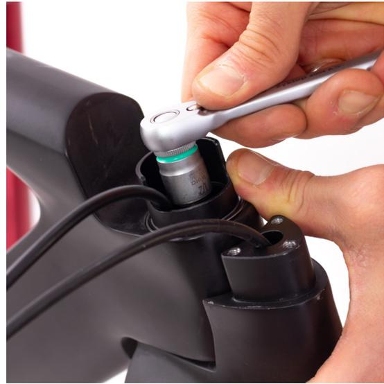
10. Slide the brake hoses through the top of the handlebar (check the hose positions in the picture).
