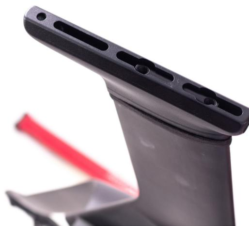
29. Place the seat post clamp on top of the rail and tighten it to 6 Nm (two bolts should align with threaded holes of the pin).
