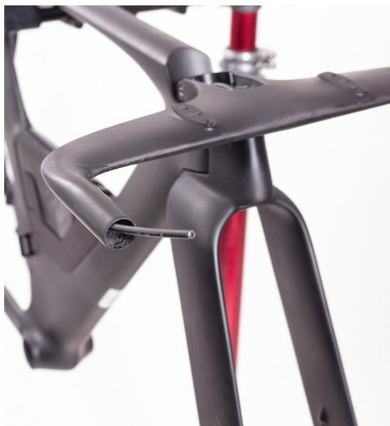
13. Tighten the handlebar to the fork using the three M5 bolts at the specified torque (6 Nm)
