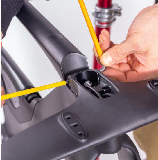
15. Afterwards, insert the handlebar top cover and tighten it to 2 Nm.
