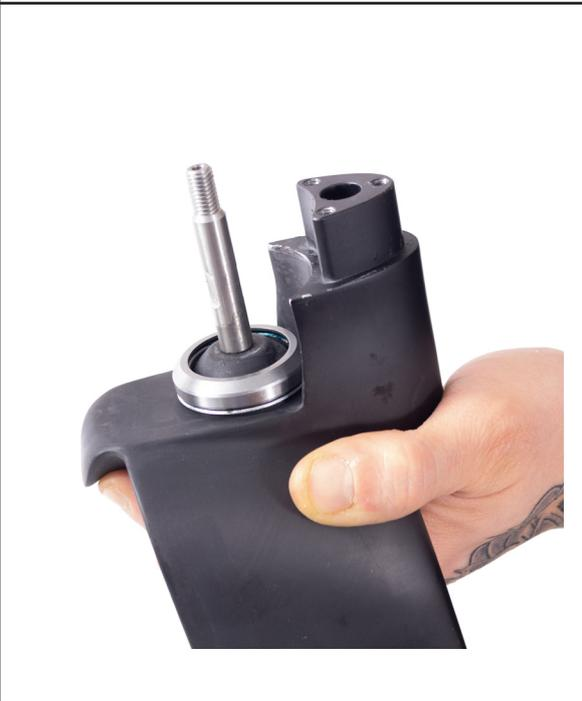
3. Insert the Anti Rotation System into the fork cone horizontally and tighten it to 5 Nm. Ensure correct alignment, as shown in the picture.
