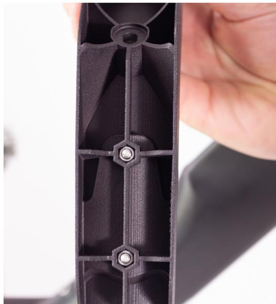
18. Place the bottle cage against the frame and tighten it to 4 Nm (the bottle cage is correctly installed when there is minimal clearance with the frame, as shown in the picture).
