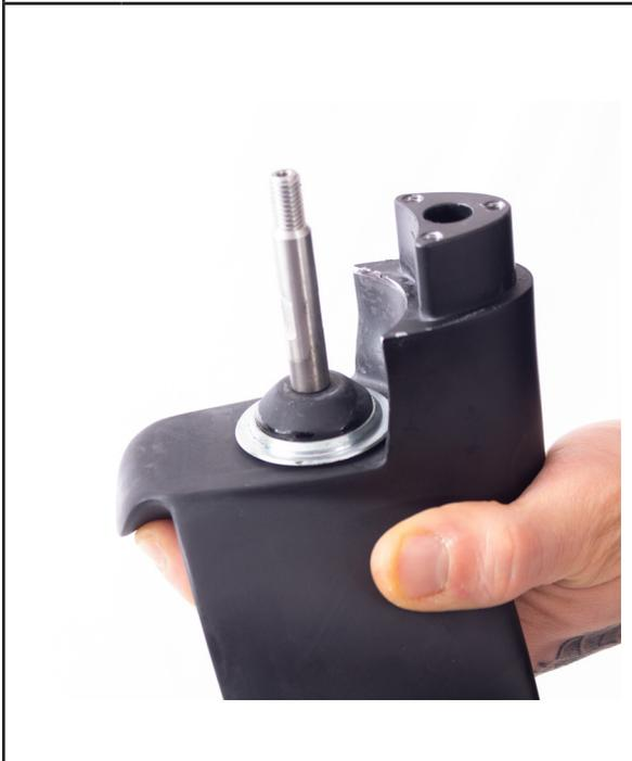
2. Insert the lower bearing in the crown race.
