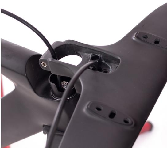
11. To make the operation easier, proceed on slightly tightening the handlebar in the fork cone.
