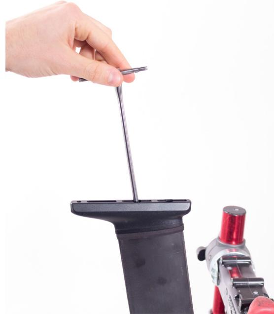
27. Insert the threaded pin into the seat post rail hole. It will be used to secure the seat clamp.
