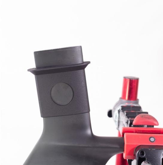
20. Lightly mark the seat tube area where the frame will be cut using a sharpened tool.
