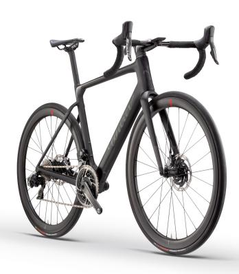
It's hard to believe that this bike hides a system providing electric pedal assist. Yet, it does. Filante Hybrid is an electric road bike that integrates the lightest pedal assist system in the world: the new X20 motor by Mahle, a German multinational that is driving technological innovation toward zeroimpact mobility.
