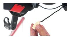
3. Connect the connector that will be connected with the iWOC button (ON/OFF switch), with a metallic wire guide, so that you can pull it out from the hole on the top tube.
