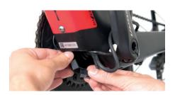
11. Fix the charging point with the tightening screws, placing the plastic cover properly.
