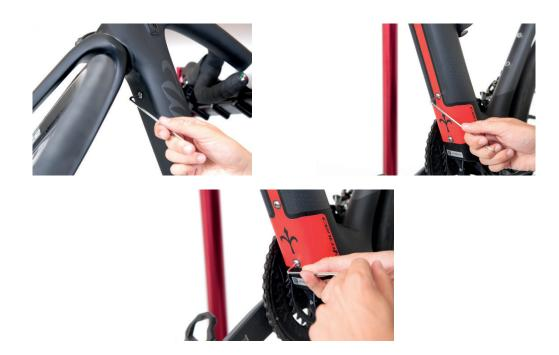
7. Connect the battery cables to the cables of the other devices (remove then the masking tape that protects the connectors).
