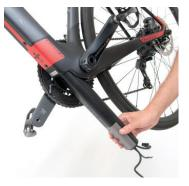
6. Tight the battery to the frame suing the screws previously disassembled (they could be stored inside the bike box). The screws must be inserted in the designated 3 points, being careful that the other internal cables pass over the battery.
