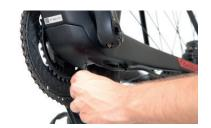
2. Protect the battery connectors with masking tape, so that you don't damage them during the assembly operations.
