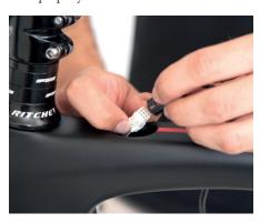
9. Install the iWOC button on the top tube, fixing it with the proper screw with a maximum torque of 2Nm.
