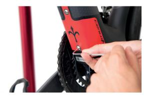
9. Remove the battery from the down tube sliding it out of the tube. Make attention to not damage the cables that pass inside the down tube.
