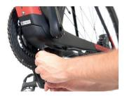
2. Disconnect the engine cable with the battery's one; follow the arrows that are placed in the insertion point. Remove the clips that fix the cable to the chain stays.
