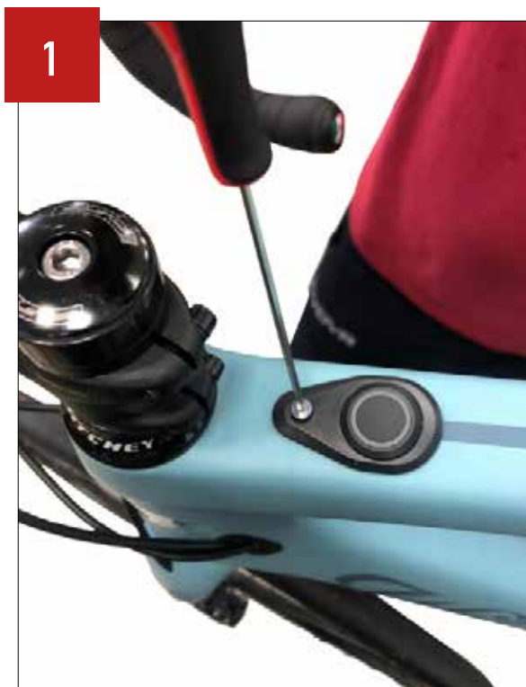
Remove the iWoc closing screw from the top tube and take the button away
