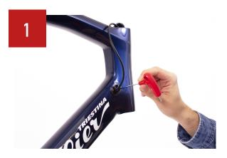
Remove the fork and the handlebar from Jena Hybrid in order to allow the following assembly operations.
