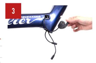
Disconnect the two cables (battery and iWoc) so that they are loose.
