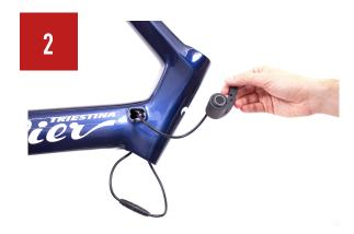
Pull out, from the lower hole of the head tube, the cable connecting the battery to the iWoc button, that are still connected together.
