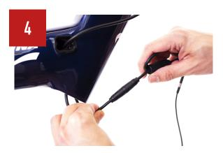
Connect the battery cable to the corresponding one of the ANT+ conversion kit (B).
