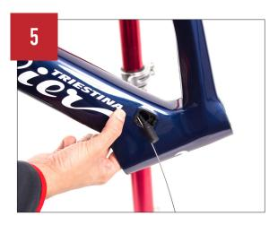
Pull out the cable fixed to the metallic guide through the side hole. Fix the battery to the frame. Screw the iwoc button to the holder with the metallic ring.
