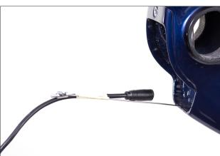
Connect the extremity of the battery/iwoc cable to the metallic guide.
