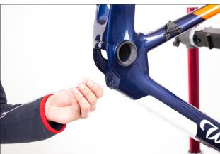
Pass a metallic guide through the side hole of the downtube until the bb.
