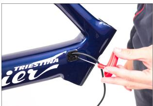
Close the side hole with the two closing metallic plates.
