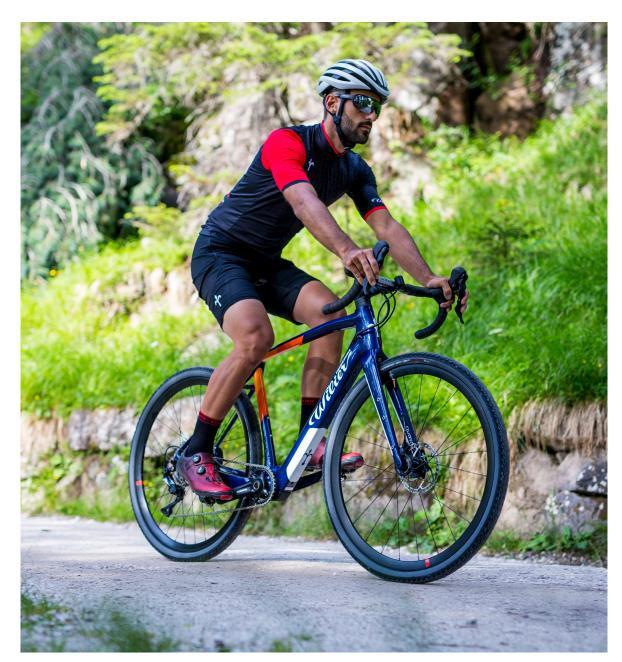
Jena Hybrid has a carbon monocoque frame and fork. The frame's geometry is similar to the Jena, offering a performance endurance ride combined with a comfortable ride position for long hours spent in the saddle.
