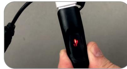
6. When the GCU led is alternating green and red, remove the GCU.
