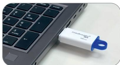
1. Connect the USB drive (FAT32, under 32GB of storage) to the PC, copy only the upgrade files in the USB.
