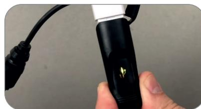
5. If the update is OK the led should be blinking in yellow (work in progress) then alternating green and red (end of update).
