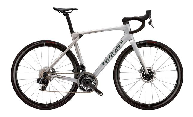
Granturismo SLR is the racing bike designed to bring out the utmost performance and comfort. With Granturismo SLR you will be able to travel long distances, minimising postural stress thanks to the special endurance geometries and to the ACTIFLEX 2.0 system, a renewed version of the rear micro-shock absorber developed in 2017 for the Cento10 NDR.
