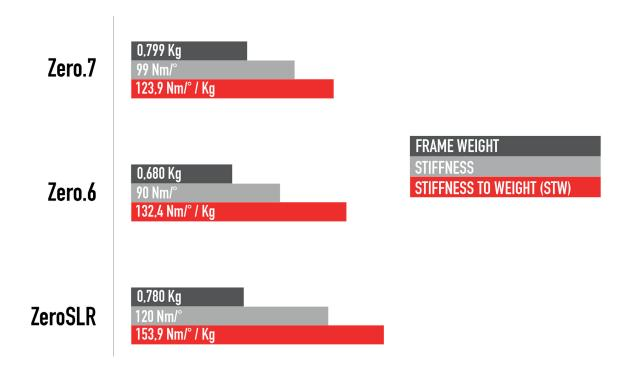
On the **ZERO SLR**, thanks to the blend of carbons, the unique positioning of the fibers and the construction technology, we have succeeded in attaining the highest level of both lightness and stiffness, exceeding the STW value of our previous Zero.7 and Zero.6 models by 24%.
