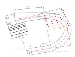
In the two figures above you see the 35 Accu-Fit points available for each frame size. The configuration on the left has no spacers, with the first size of stem. Also the configuration on the right has the first stem size but with all the spacers installed.
